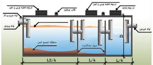
Grease trap or grease trap is a device made of fiberglass, concrete, polyethylene and composite with a capacity of 200 liters to 50 cubic meters. Degreasers are responsible for waste products from washing dishes and cooking and prevent clogging of sewer pipes and endangering the sewer system.
